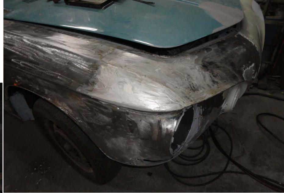
The finishing work is done with molten tin, not bondo filler, just as the Karmann coachbuilders did it in the 1960's. The joined edges are filled with molten tin and paddled into shape to match the contours. Then a flat file is used to remove the excess tin, making the panel smooth & straight. This tin work is a real lost art that most body shops will not even attempt to do when replacing metal panels on an old car.
