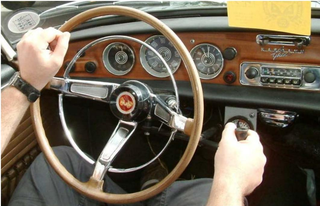
The special steering wheel was one of the original options as was the AM/FM radio, and the Eberspacher gas heater. The heater's 24-hour timer dial is located under the dash to the left of the ash tray. The electrically-heated rear window option has a warning light in the dash just above the clock. Dave is handicapped so he had a manual braking & acceleration apparatus fitted (which will be removed once it's sold).
