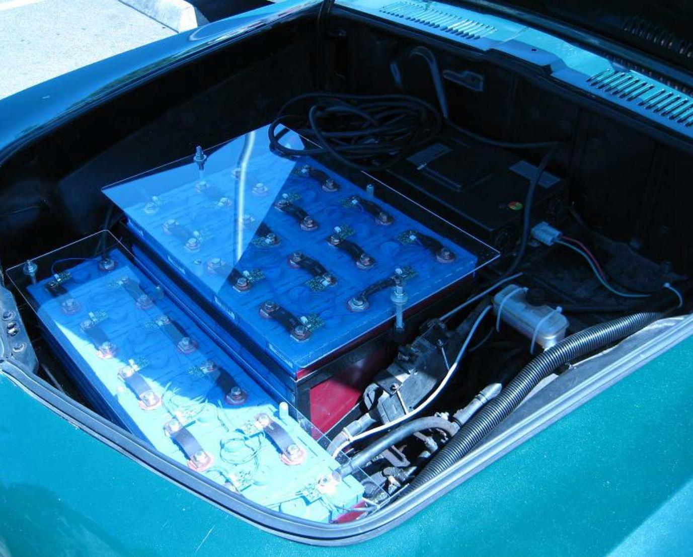
Here's the money shot: front compartment filled with 24 cells, battery management cell boards, and a 120V charger. The rear compartment has the motor, motor controller and 240V charger. All of these electric parts are neatly hidden from the outside, retaining the styling of the T34's classic 1960's body lines.
