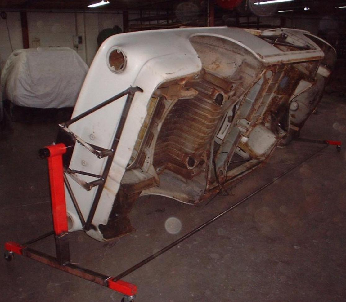
Where to start? I thought replacing the panel above the transmission would be a decent place to start so in order to get at it properly the parcel shelf needed to come out so I got to work drilling spot welds out (below). You can see the heavily rusted C-pillar and the rusty seams between the panels behind the rear seat.
