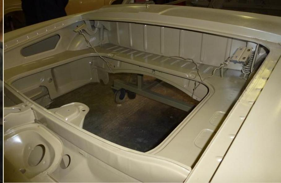
These photos were taken after the triple-series of chemical dipping to remove the paint, rust, & apply the anti-rust coating of primer paint. You can see the original tin, used to join the metal panels at the Karmann factory, has been removed, so these seams will be finished-off next. This dipping process is essential to be confident all of the rust has been removed forever.
