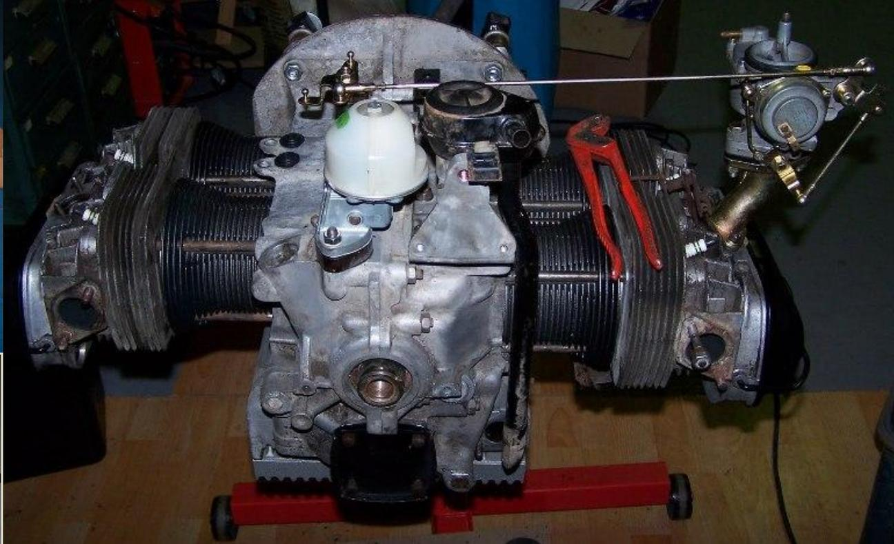
I also had all of the non-chrome metal parts galvanized including the door window regulators, screws, & bolts. Black powder-coating was applied to the engine sheet metal and spare tire carrier. The fuel tank was rusty so it was de-rusted first and then coated with a plastic solution inside. The engine was rebuilt & reassembled. It's nice to see these old parts new once again!"
