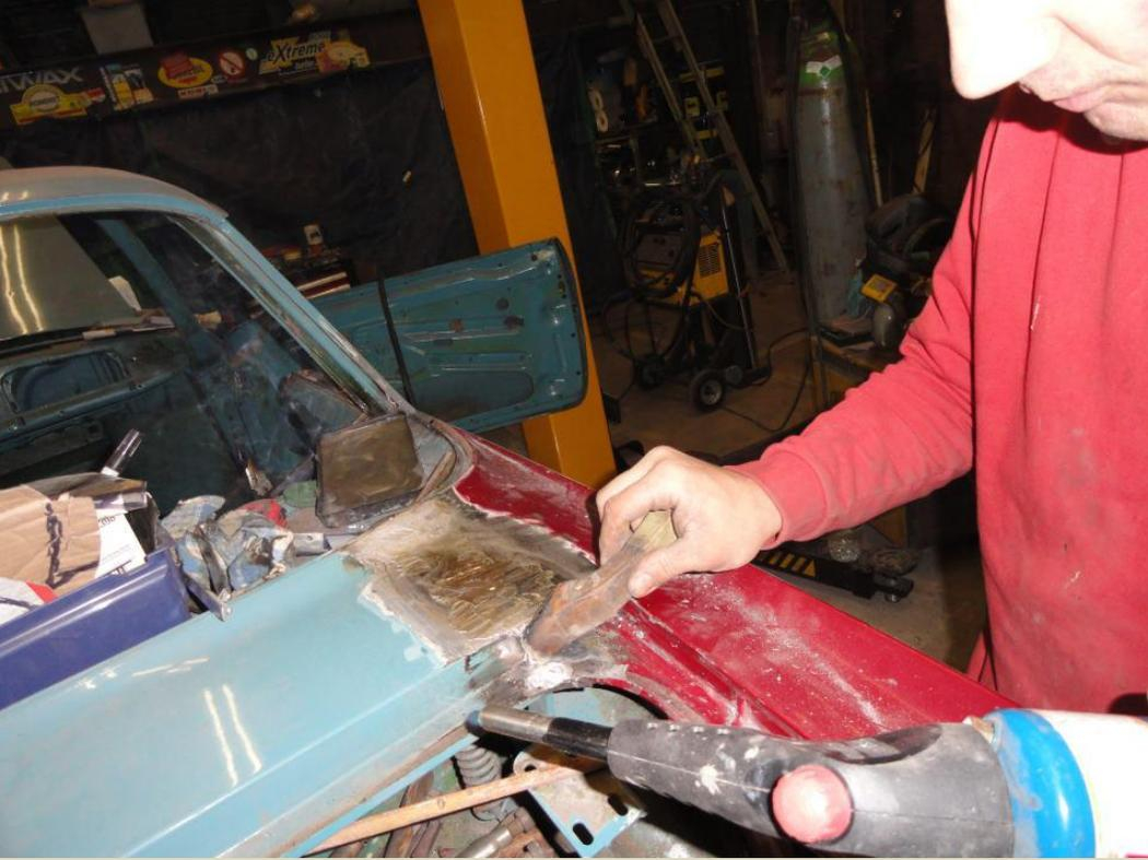
You can see the left-rear fender metalwork in bare-metal form after the wheel arch was welded into place and a hand-formed lower rear corner section was created by Jurgen. The lower-left photo shows Chris drilling-out the weld spots along the left rocker panel area.
