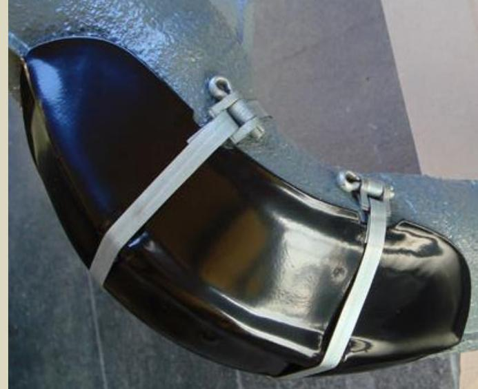
Position the shield & straps loosely. Originally VW had the clamps on the inboard sides. The strap wraps around the heat exchanger once, threads through the rectangular hole on the clamp, then wraps around a second time and threads through the cotter key. Pull in the slack and then trim off some of the excess strapping. Then tighten the key with a screwdriver a half-turn at a time, stopping to adjust the strap and reposition as necessary as you go. Turned out very nice!
