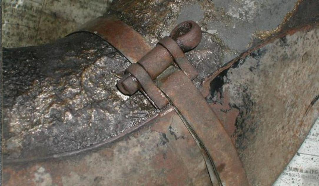
I did some research on substitutes for the coating and settled on Lizard Skin ([www.lizardskin.com](http://www.lizardskin.com)) ceramic insulation. It's not cheap but it has properties that make it a good choice for the job: good heat & sound insulation, withstands temperatures to 500°F, water based & non-toxic. I applied it with a brush over ISP West's ceramic coating, recreating the original texture, and then gave it several coats of engine enamel.
